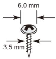
Do not drive the screws in all the way into the wall—leave a space of about 2 mm to allow room for sliding the wall-mount panel between the wall and the screws.
