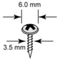
Do not drive the screws in all the way into the wall—leave a space of about 2 mm to allow room for sliding the wall-mounting panel between the wall and the screws.
