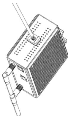
**STEP 1:** Screw the cable holder onto the bottom of the AWK-3131.
