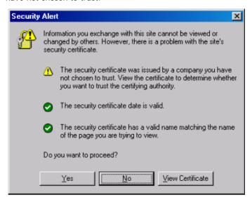
3. Select Yes to accept the certificate issued by Moxa IW and then enter the AWK-3131-M12-RCC's web browser interface secured via HTTPS/SSL. (You can see the protocol in URL is https.) Then you can use the menu tree on the left side of the window to open the function pages to access each of AWK-3131-M12-RCC's functions.
