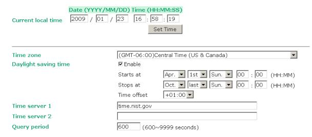
The *Current local time* shows the AWK-3131-M12-RCC's system time when you open this web page. You can click on the **Set Time** button to activate the updated date and time parameters. An "(Updated)" string will appear to indicate that the change is complete. Local time settings will be immediately activated in the system without running Save and Restart.
