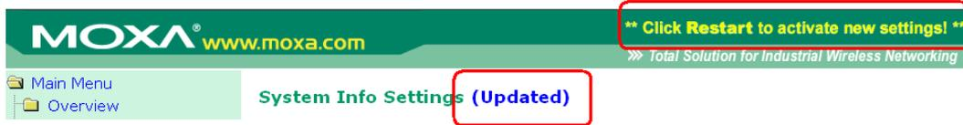
To activate the changes click **Restart** and then **Save and Restart** after you change the settings. About 30 seconds are needed for the AWK-4131 to complete the reboot procedure.
