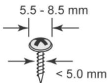
Do not drive the screws in all the way into the wall—leave a space of about 2 mm to allow room for sliding the wall-mounting kit between the wall and the screws.
