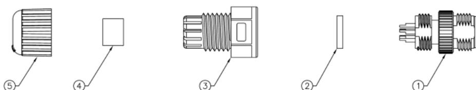
1. Refer to the pin assignment and solder wires with ①;
