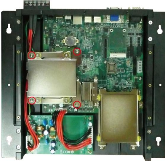
2. Remove two black screws on each side of the bracket, and then take off the cover.
