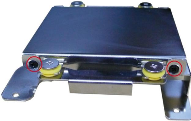
3. Place the hard disk on the bracket. Use the four screws to fasten the hard disk at both sides of the bracket.
