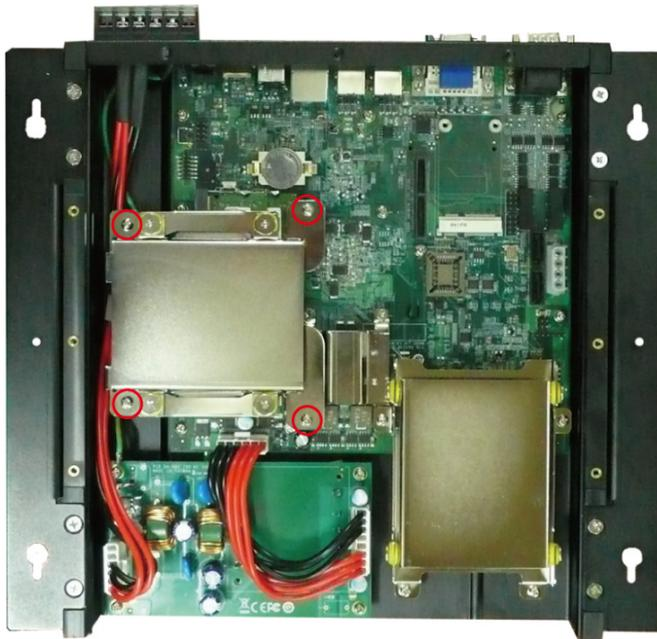
7. After the first HDD bracket has been removed, you can find two memory modules. Carefully remove the module by clicking the clutches at both sides of the module, and then replace the new module. Be sure to orient the module correctly.
