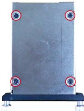
4. Place the drive into the tray and secure it in place using the four screws. When finished, insert the tray into the computer and fasten the tray in place using the two thumbscrews on the front panel. Finally, complete the installation by turning the key leftwards to lock the tray into place.
