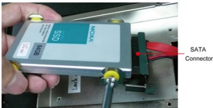
4. Replace the storage drive into the computer and secure it using the four mounting screws you removed in step 1.
