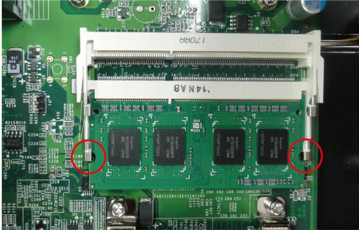
5. Carefully slide the module into the clutch at an angle, and then push downward. Make sure the module has been firmly inserted and is oriented correctly.
