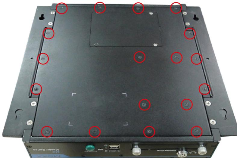
2. Remove the removable storage tray on the front panel of the computer, and then remove the bottom cover. Then you need to remove four screws on the storage tray.
