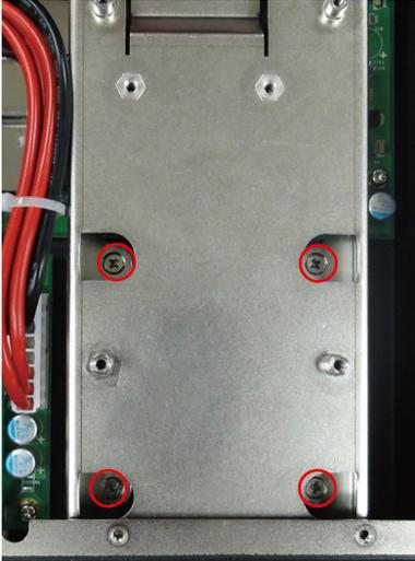
3. When finished, remove the storage tray, and you can see the location of the memory module.
