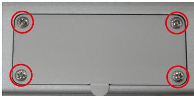
2. Remove the SSD by pulling out the plastic plate (shown at left).
