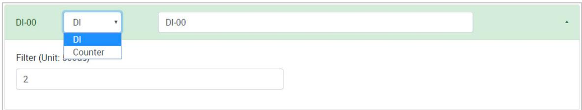
**Channel Mode Drop-Down List:** It lists all of the channel modes, which can be operated by this channel. Select **DI** or **Counter** mode for each channel (option: DI or Counter).
