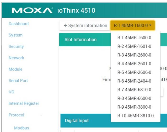
**Locate:** Identify the physical location of the module and the module’s status LED will blink green.
