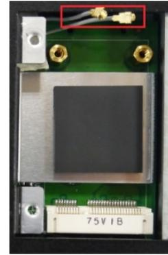
2. Insert the cellular module into the socket and fasten two screws (included in the package) on to the top of the module. We recommended using a tweezer when installing or removing the module.
