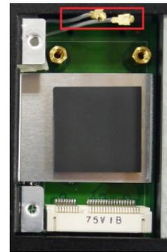
2. Insert the Wi-Fi module into the socket and fasten two screws (included in the package) on to the top of the module. We recommended using a tweezer when installing or removing the module.
