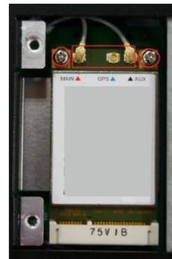
5. Connect the cellular antennas to the connectors. Antenna connectors are located on the front panel of the computer.
