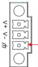
Connect the 9 to 48 VDC power line to the terminal block, which is connector to the UC-5100 Series computer. If the power is supplied properly, the "Power" LED will glow a solid green light. The power input location and pin definition are shown in the adjacent diagram.
