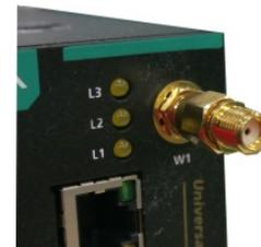
6. Connect the Wi-Fi antennas to the antenna adapters.
