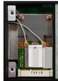
5. Connect the antenna adapters to the connectors on the front panel of the computer.
