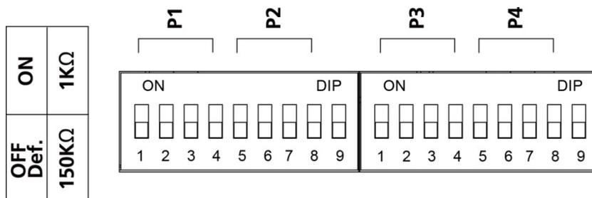
Each port consists of 4 pins; you must switch all 4 pins of a port simultaneously to adjust the value of the port.
