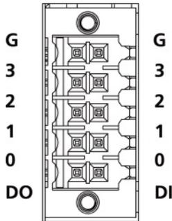
The UC-5100 Series comes with 4 digital inputs and 4 digital outputs. The DI/DO connectors are located on the top panel of the computer. Refer to the diagram on the left for the pin definitions. For the wiring method, refer to the following figure:
