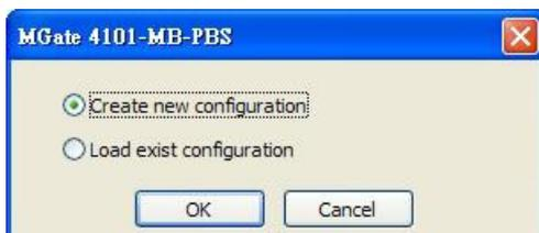
By choosing "create new configuration," users can set each functions as online setting. Refer to the **Modifying the Configuration** section for detailed information. When all configurations are finished, click **OK** to update or store the configuration file.
