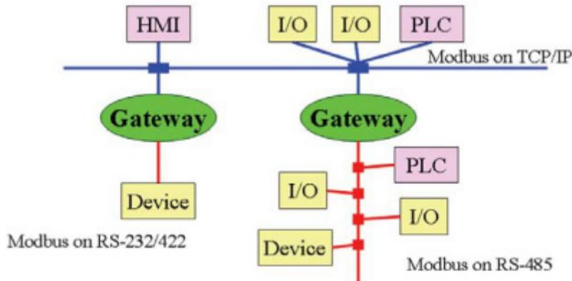
Ordinarily, Modbus TCP and Modbus ASCII/RTU are unable to communicate with each other.
