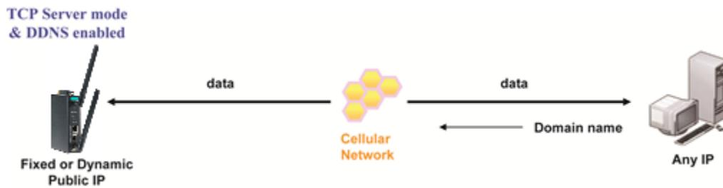
**Connecting TCP client and TCP server within the same cellular service provider**
