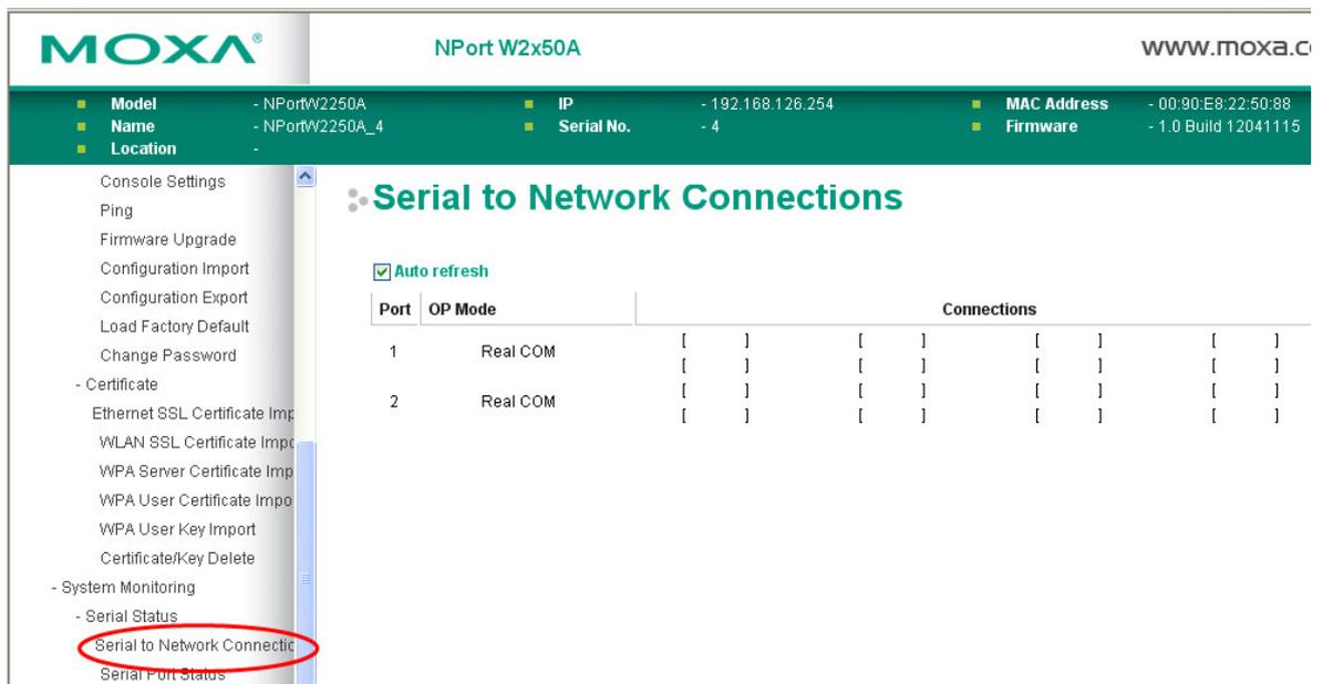
The **Serial to Network Connections** page is located under **Serial Status** in the **System Monitoring** folder. On this page, you can monitor the current operation mode and host connection status for each serial port.
