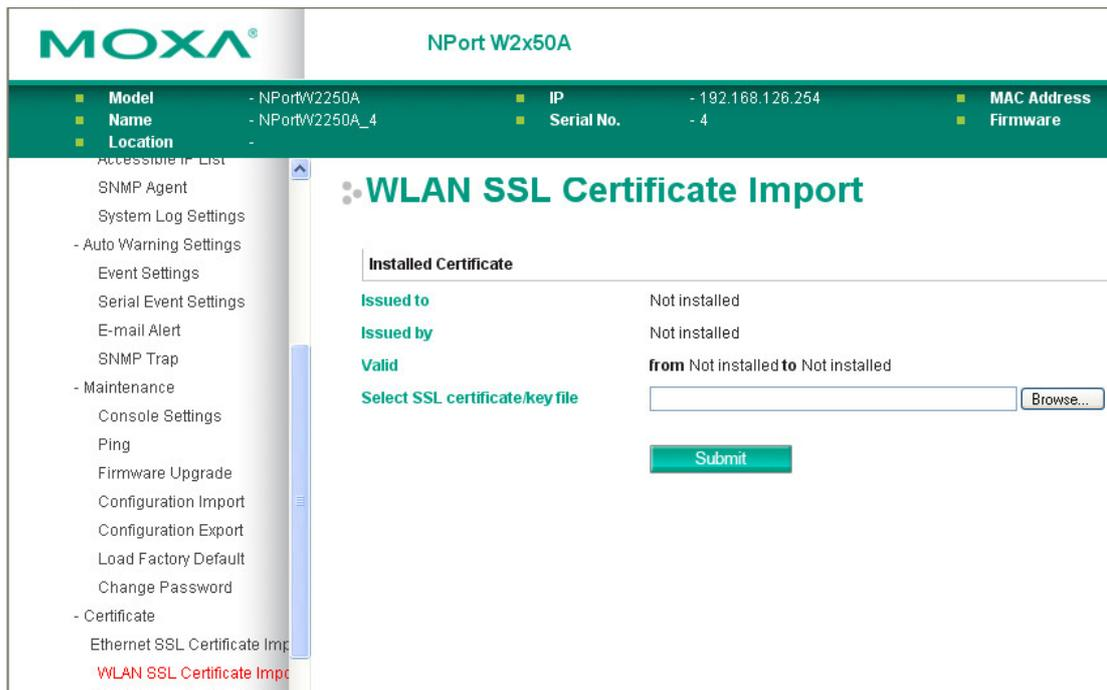
The **WLAN SSL Certificate Import** page is located under **Certificate** in the **System Management** folder. By default, the WLAN SSL certificate is automatically generated by the NPort based on the IP address of the wireless interface. You can also import a certificate. Select or browse for the certificate file in the **Select SSL certificate/key file** field.
