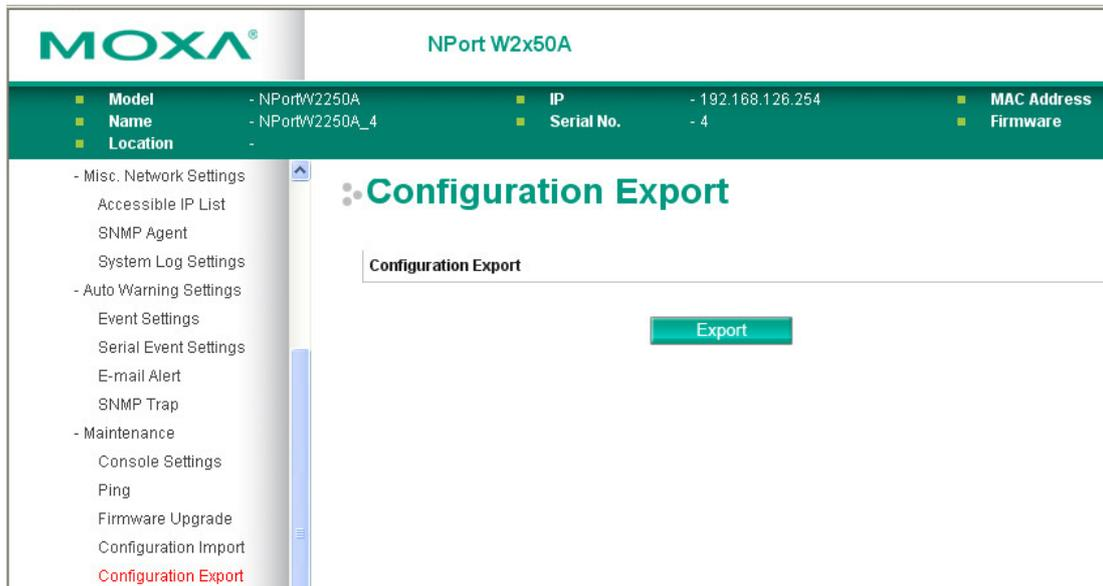
The **Configuration Export** page is located under **Maintenance** in the **System Management** folder. This is where you can save the NPort's current configuration to a file on the local host. Click **[Download]** to begin the process. A window should appear asking you to open or save the configuration text file.
