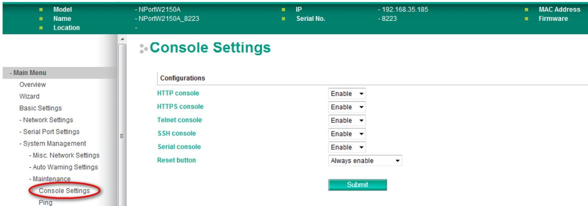
The **Console Settings** page is located under **Maintenance** in the **System Management** folder. This is where you enable or disable access to the various NPort configuration consoles, as well as the behavior of the reset button. You may modify **HTTP console**, **HTTPS console**, **Telnet console**, **SSH console**, **Serial Console**, and **Reset button**.
