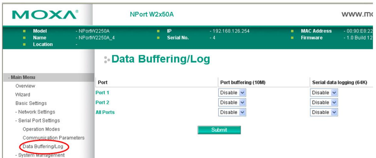
On the serial port's **Data Buffering/Log** page, you can enable or disable **Port buffering** and **Serial data logging**.
