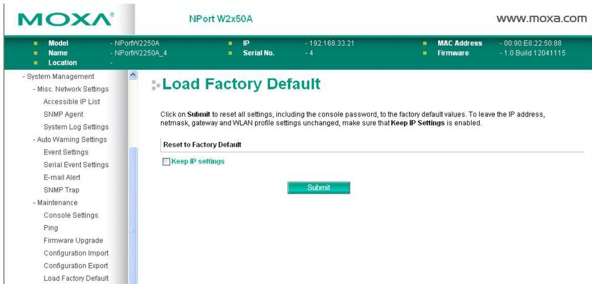
The **Load Factory Default** page is located under **Maintenance** in the **System Management** folder. Click **[Submit]** to reset all settings to the factory defaults. You can preserve the NPort’s existing IP settings (i.e., IP address, netmask, gateway, WLAN profile, and all certificates) by making sure that **Keep IP settings** is checked before clicking **[Submit]**.
