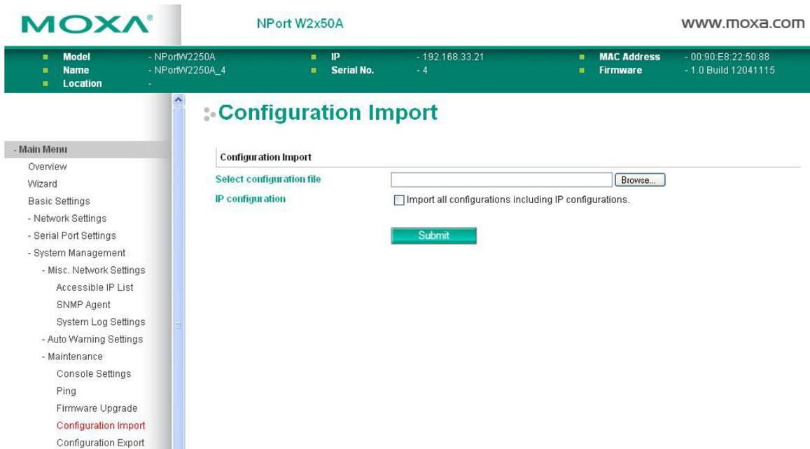
The **Configuration Import** page is located under **Maintenance** in the **System Management** folder. This is where you can load a previously saved or exported configuration. Select or browse for the configuration file in the **Select configuration file** field. If you also wish to import the IP configuration (i.e., IP address, netmask, and gateway), make sure that **Import all configurations including IP configurations** is checked.
