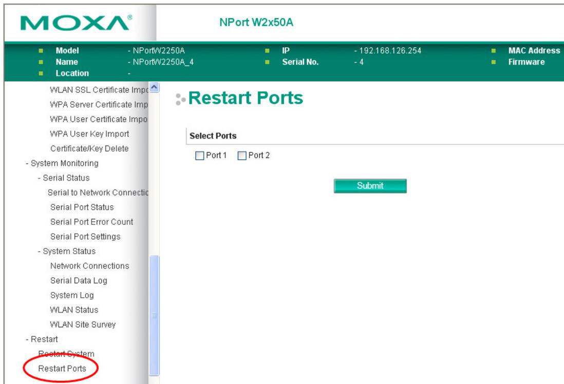
The **Restart Ports** page is located in the **Restart** folder. Select the desired serial and click **[Select All]** to select all serial ports. Click **[Submit]** to restart the selected serial ports.
