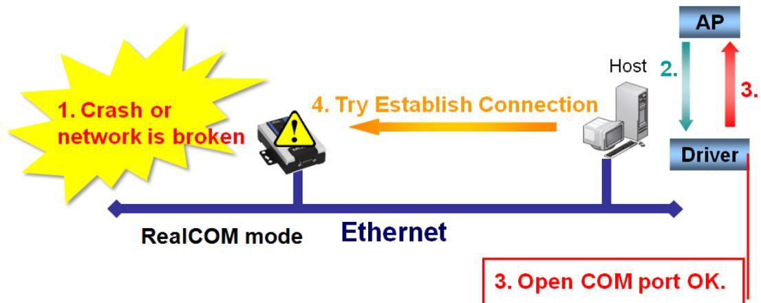
**Drop Writing Data if Network Connection is Lost:** This function will assure the data to be kept in the buffer or dropped when network connection is lost. The buffer size is 4 KBytes.
