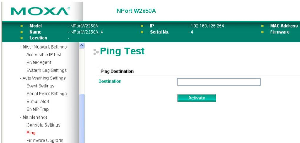
The **Ping** page is located under **Maintenance** in the **System Management** folder. It provides a convenient way to test an Ethernet connection or verify an IP address. Enter the IP address or domain name in the Destination field and click **[Activate]**. The results will be displayed immediately.
