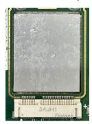
2. Place the thick thermal pad on the heat sink.
