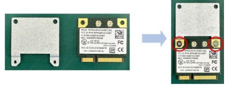
2. Find the slot 4 and place the thick thermal pad close to the slot like picture below:
