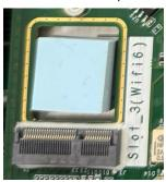
2. Unfasten the screw and insert the module into the socket above the thermal pad.
