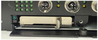
5. Push the clutch in the tray to the left to make sure the disk drive has been connected correctly.
