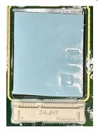
3. Unfasten the screw and insert the module into the socket above the thermal pad.
