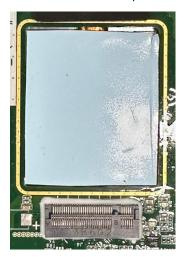
2. Unfasten the screw and insert the module into the socket above the thermal pad.
