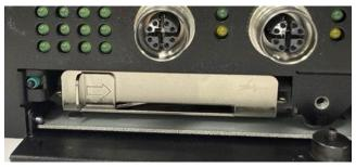
6. To remove the tray, pull the clutch in the tray to your right and pull out the tray.
