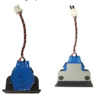
Reconnect the connector, place the battery holder into the slot, and secure the cover of the slot by fastening the two screws on the cover.
