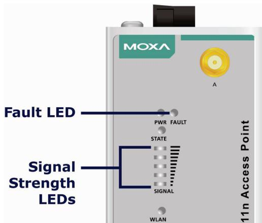
The following table summarizes how to read the device's wireless settings from the LED displays.
