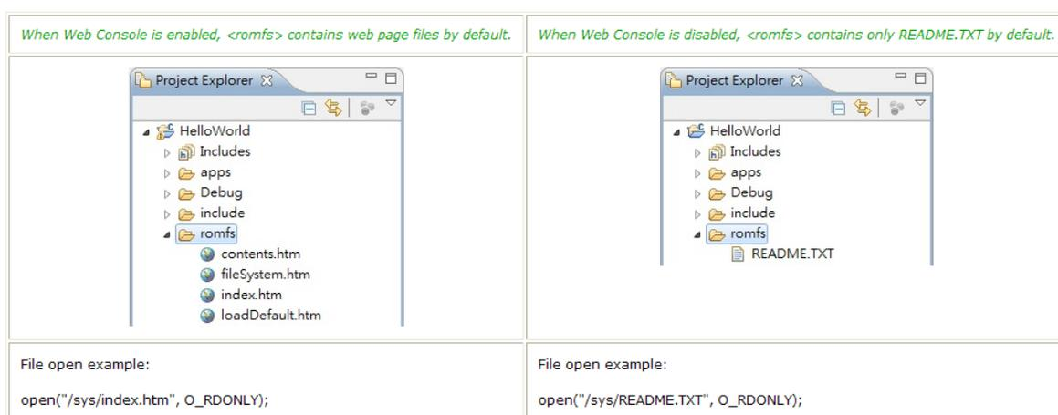
All files in <romfs> directory will be compiled into ROM file system of MiiNePort-SDK. The files in ROM file system are available through the mount point "/sys". The maximum storage size of ROM file system is 512K bytes.
