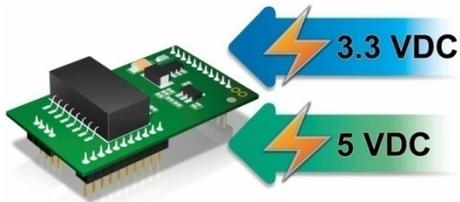
The **EZPower** function makes it easy to configure the MiiNePort's input voltage. Use EZPower to configure the MiiNePort's system power input to either 3.3 VDC or 5 VDC.
