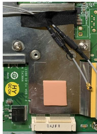
4. Install the Mini PCIe half-card fix board and secure it with the two silver screws (M2.5 x 6 mm).
