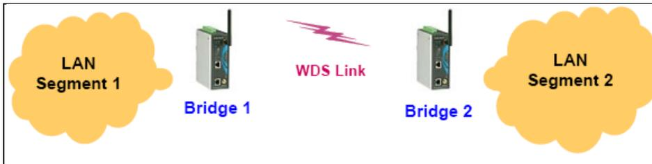
It is a good idea to plan your wireless network by drawing a diagram so that you know how each AWK-4131A is connected to other peer APs or wireless bridges by WDS, and how bridges are connected to other peer bridges by WDS. See the following figure for an example of a network-planning diagram.
