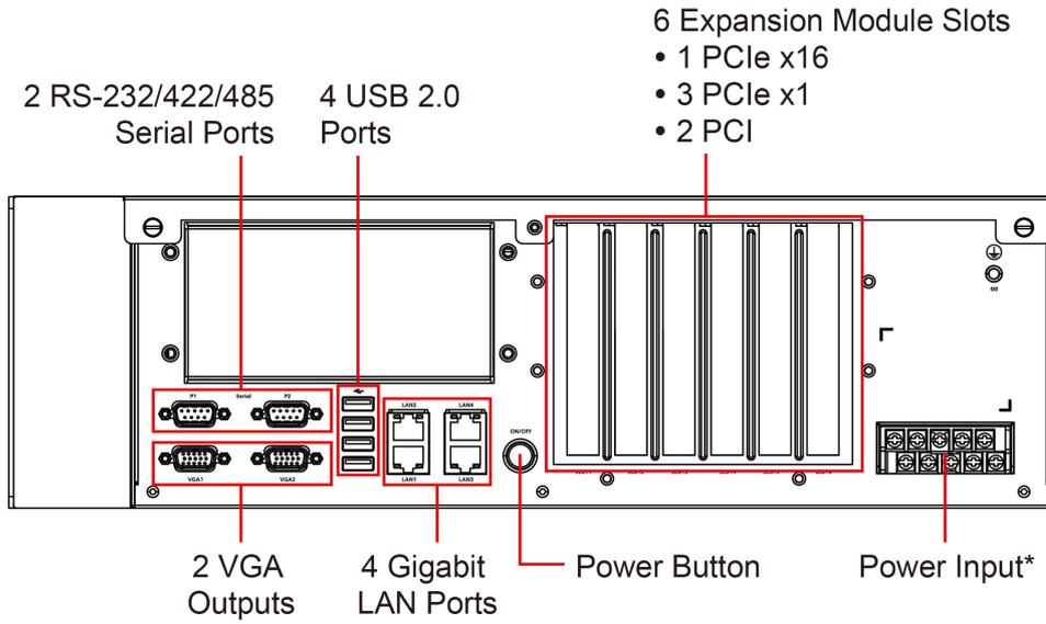
\*The power input supports two types of power supply (refer to the section "Connecting the Power" in Chapter 2 for details):
