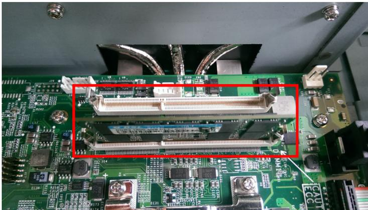
4. If a memory module is already installed in the socket, push the two fasteners to free and then remove the module. Insert the new memory module into the socket, making sure you insert the SDRAM in the correct direction. Push down the memory module, making sure that the two fasteners snap in place and are holding the module firmly.
