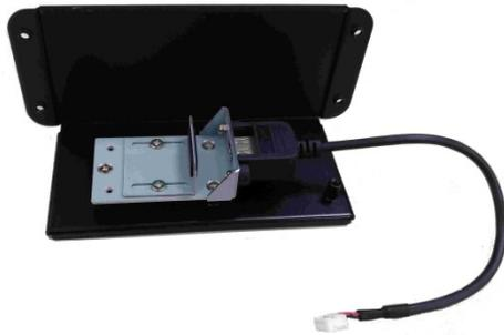
3. Plug your USB dongle into the USB port of the dongle bracket.
