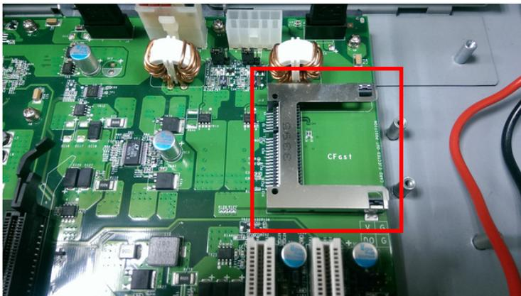
4. Insert the CFast card into the socket.
