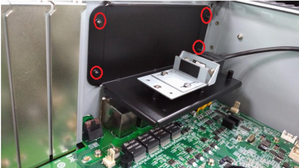
The USB Dongle Kit should be installed as close to the memory socket as possible as shown in the following image:
