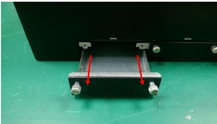
**Step 3:** Place the SSD/HDD in the tray as shown, and then flip the tray over to fasten the screws.
