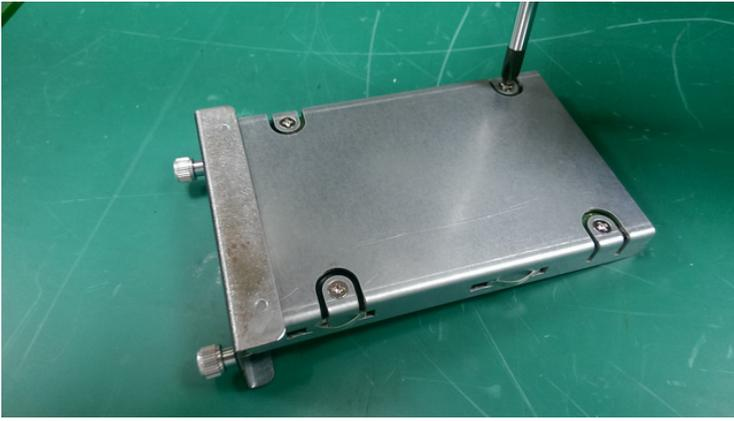
**Step 4:** Insert the SATA Tray into original SATA slot and fasten the screws.
