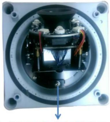
2 screws for fixing the lens in a horizontal position (5.5 kgf-cm)
