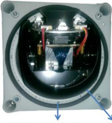
Calibrator for tuning the lens in a horizontal position (0 to 350°)
