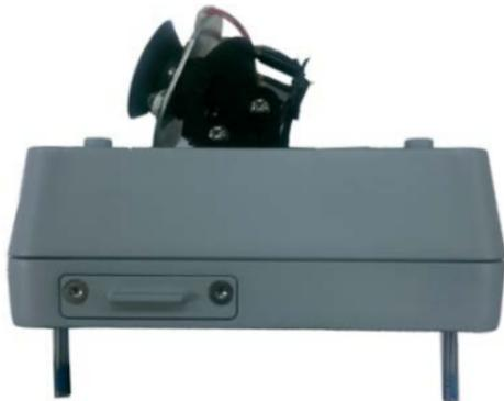
**Step 6: Stick the dry packs into the camera. Stick the double-sided tape on the dry pack, and then stick the dry packs on the location shown in the picture.**
