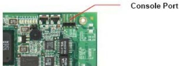
Serial Console Port & Pinouts
