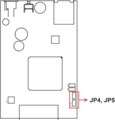
Jumpers are used to set the pull high/low resistors. The default is 150 kΩ. Short the jumpers to set this value to 1 kΩ. Do not use the 1 kΩ setting with RS-232 mode, since doing so will degrade the RS-232 signals and shorten the communication distance.
