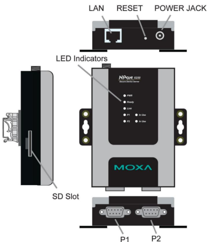
**Reset Button**—Press the Reset Button continuously for 5 sec to load factory defaults. Use a pointed object, such as a straightened paper clip or toothpick, to press the reset button. This will cause the Ready LED to blink on and off. The factory defaults will be loaded once the Ready LED stops blinking (after about 5 seconds). At this point, you should release the reset button.
