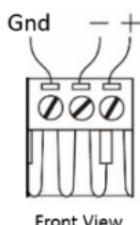
**STEP 1:** Insert the negative/positive DC wires into the V-/V+ terminals, and the ground wire into the GND terminal.
