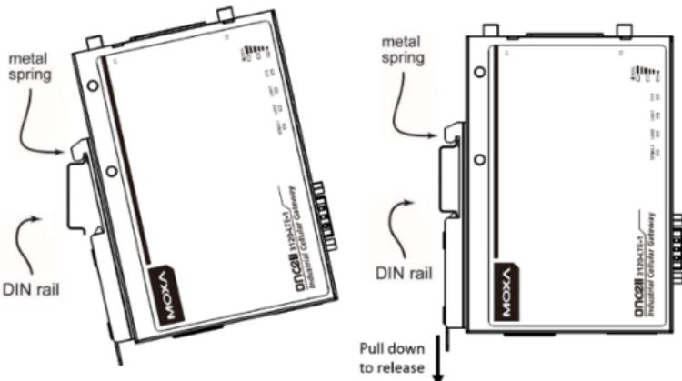
To remove the OnCell 3120-LTE-1 from the DIN rail, pull down the lever at the bottom of the DIN-rail kit.
