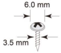
**NOTE** Before tightening the screws into the wall, make sure the screw head and shank size are suitable by inserting the screw through one of the keyhole-shaped apertures of the Wall Mounting Plates.
