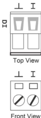
**STEP 1:** Insert the negative (ground)/positive DI wires into the  $-/+$  terminals, respectively.
