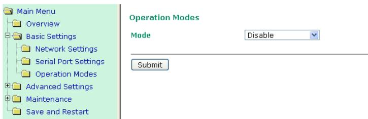
When **Mode** is set to **Disable**, that particular port will be disabled. Check **Apply the above settings to all serial ports** to apply this setting to all ports.
