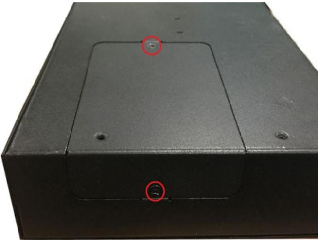
2. Remove the cover to access the SD-card slot and the mSATA
