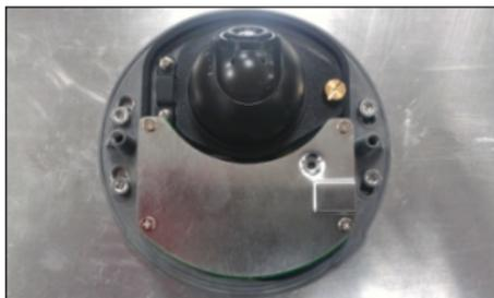
**NOTE** The screw hole for mounting the VP-FP1 fixed plate is a countersunk hole with 5 mm diameter, and 90° 2 x 2 mm chamfer. Take this into consideration when drilling these 2 screw holes.
