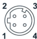
**NOTE** To connect the VPort P06-1MP-M12 to a network, use an Ethernet cable with D-code M12 connector and an M12 PoE switch or RJ45 PoE switch
