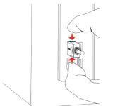
Step 2: Unplug and pull out the cable 90 degrees horizontal to the USB socket.
