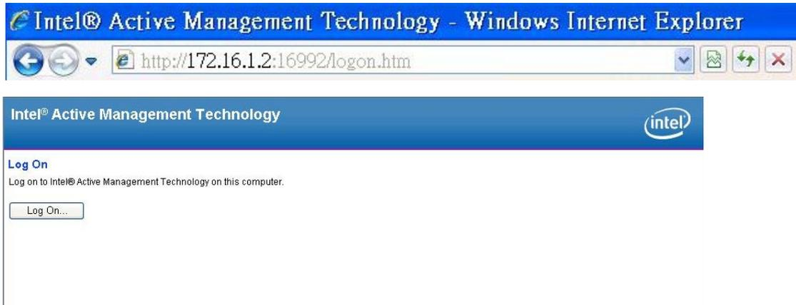
2. Click on "Log On" and type the username (**admin**) and password to log in and control the V2403C remotely.
