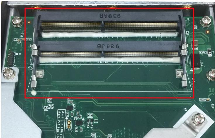
3. Insert the new memory card into the first slot, pull in the clutches, and push down the memory card. Ensure that the memory card is securely inserted.
