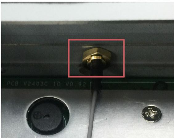
3. On the other end of the connector, pass the antenna mount's threaded connection ring through the mounting hole, hold the locking washer against the rear panel and secure the antenna connector by tightening the nut onto the threaded protection ring.
