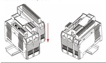
**NOTE** After the module is firmly attached to the DIN rail, the module connections to the internal bus will be established.
