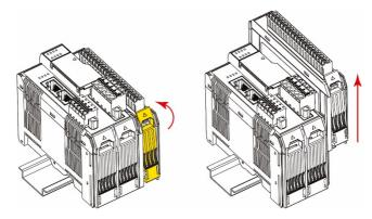
**NOTE** Electrical connections for the internal bus will be disconnected when removing the 45M module.
