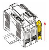
$\mbox{\bf Step 2:}$  Push the top of the release tab to latch it, and then pull the module out.
