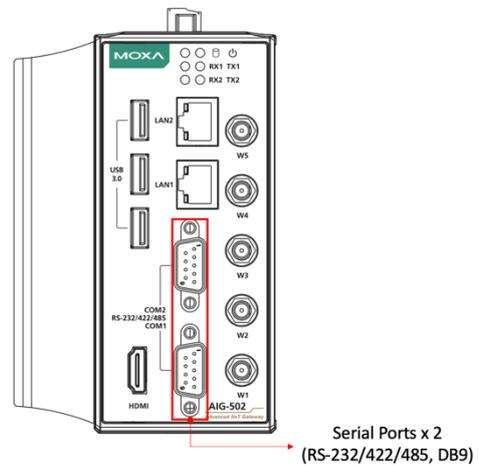
The pin assignments of the serial ports are shown in the following table:
