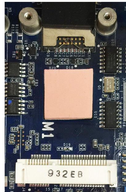
4. Insert the Wi-Fi module (with the mounting plate) into the socket and fasten the two black screws on the mounting plate to secure it.
