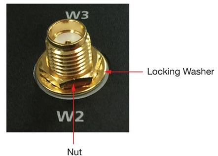
7. Connect the Wi-Fi antenna to the connector on the front panel.
