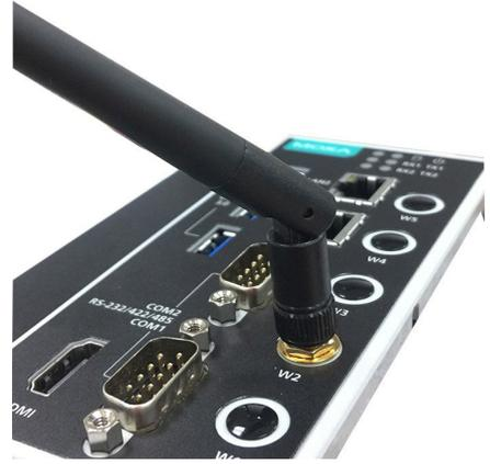
The pre-built cellular module comes with three connectors for a GPS antenna (W4), a primary cellular antenna (W3), and a secondary cellular antenna (W1).
