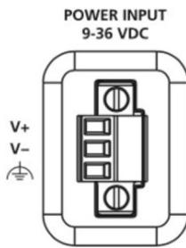
Use an LPS (9-36 VDC) or Class 2 power cord to connect to the AIG-502's terminal block to power jack converter and then turn on the power. If the power is supplied properly, the Power LED will light up. The OS is ready when the Power LED is solid green.
