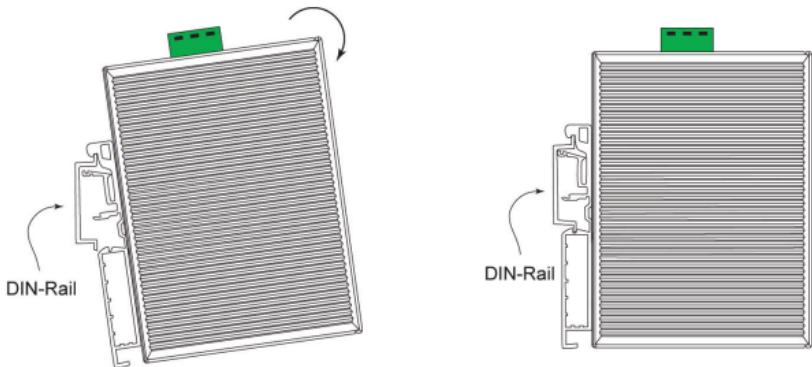
To remove Moxa EDS-208 from the DIN-Rail, insert a flat-blade screw driver horizontally into the DIN-Rail kit under the EDS-208, and then pull it upwards and release EDS-208 towards you away from the DIN-Rail.
