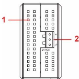
1. Heat dissipation orifices
