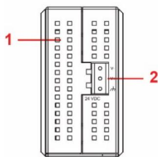
1. Heat dissipation orifices
