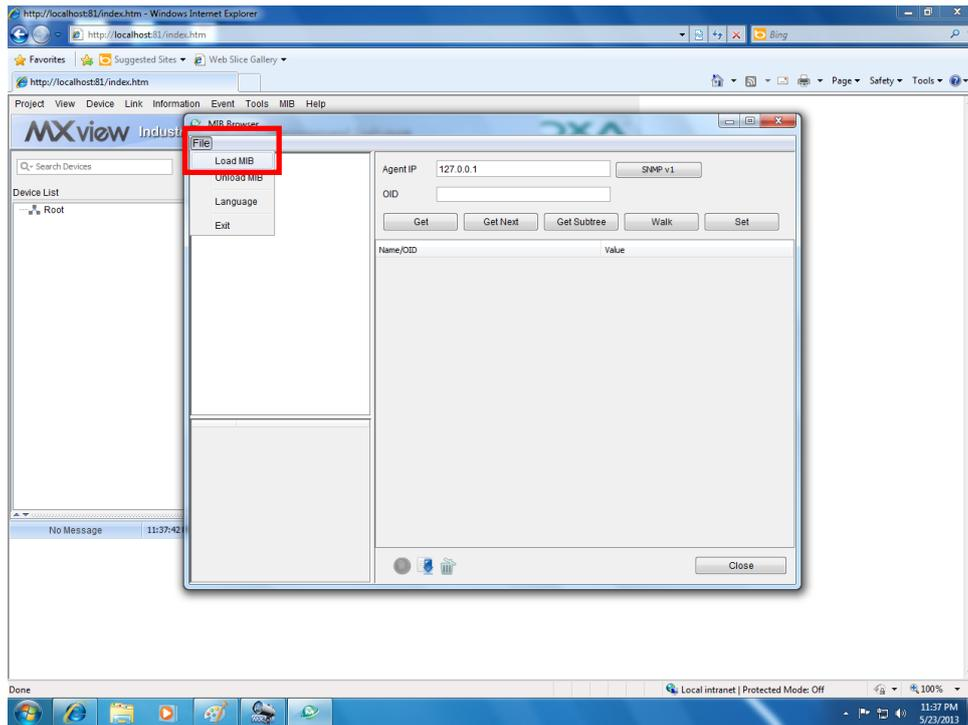
7. Navigate to **c:\usr\share\snmp\mibs\MOXA-SYS-MIB-TPMRT.txt**.
