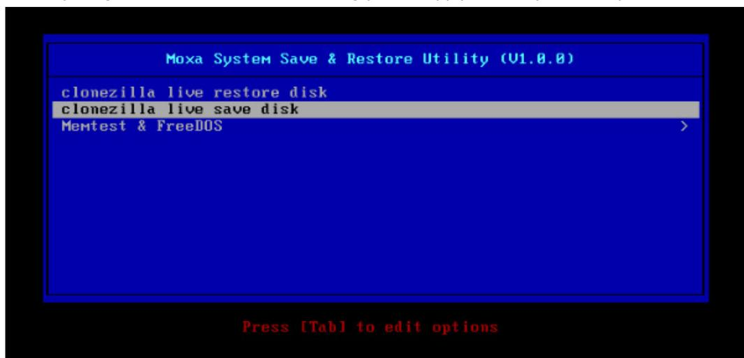
2. The V2616A will now boot into the image creation environment. Wait until the boot process has finished.
