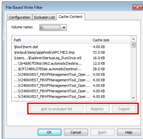
2. The most common usage of the Cache Content filter will likely be to permanently write content to the hard drive. To do this, select the file you wish to write to permanent memory and click on the **commit** button. This will delete the file from the cached overlay and replace the current file in permanent storage with the modified cache file.
