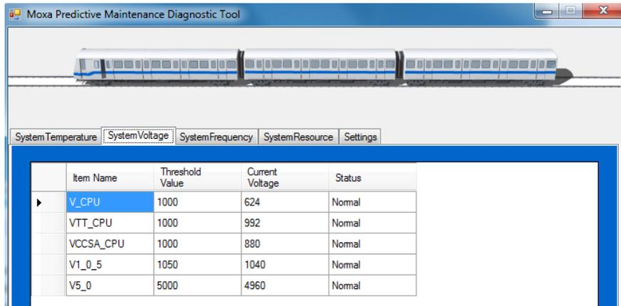
**NOTE** V\_CPU = Voltage for processor core
