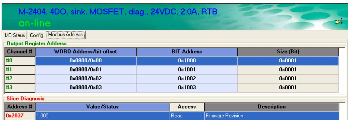
The screenshot shows the ioAdmin software interface for an M-2404 module. The top bar displays the module name and status: "M-2404, 4DO, sink, MOSFET, diag., 24VDC, 2.0A, RTB on-line". Below this, there are tabs for "I/O Status", "Config", and "Modbus Address". The "Modbus Address" tab is active, showing a table titled "Output Register Address".
