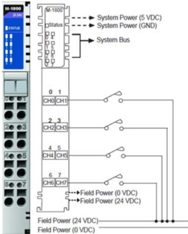
**M-1801: 8 digital inputs, source type, 24 VDC**
