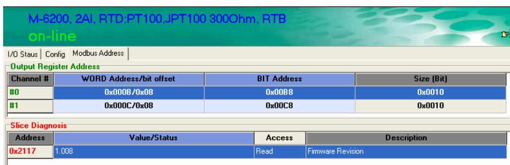
The RTD module supports different kinds of temperature sensor. To configure the sensor type, click on **config**.
