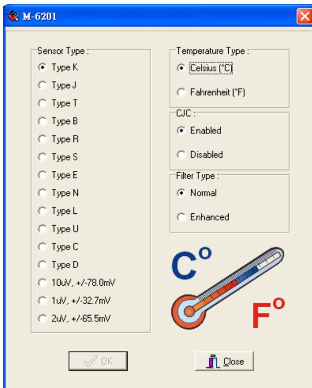
On this page, you may set up the sensor types and the temperature unit. Note that the configuration applies to all channels in the same module. The related model is M-6201.
