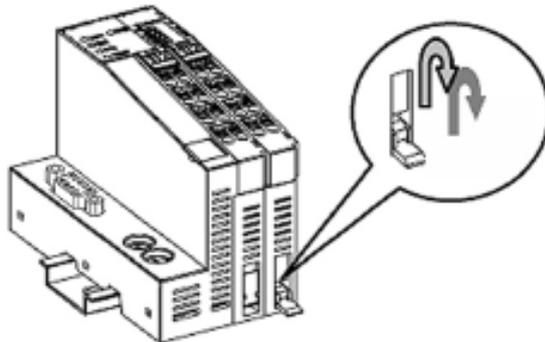
**Step 2:** Pull out the I/O module.
