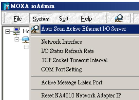
ioAdmin can automatically allocate available COM ports on the host computer and scan Unit IDs from 01 to 99 for each COM port. However, it takes longer to finish the process. A more efficient and faster method is to select **Only Search: COMx** and search designated COM ports. Note that ioAdmin supports Modbus/RTU. In a Modbus/ASCII environment, configure the Network Adapter using Modbus/RTU, and then switch back to Modbus/ASCII for field operation.
