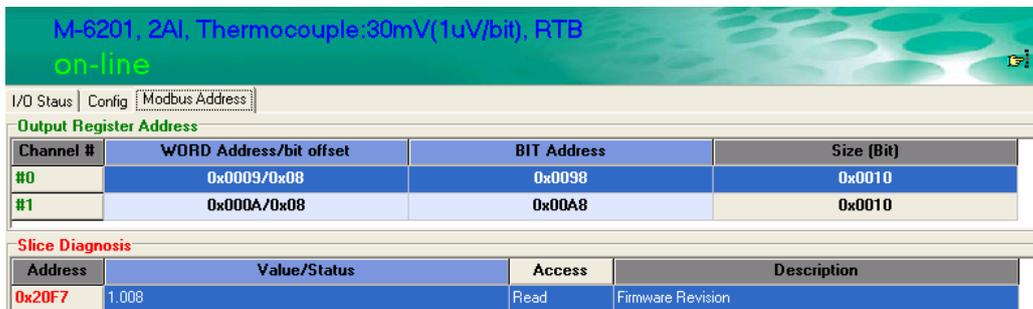
The thermocouple module supports different kinds of temperature sensor. To configure the sensor type, click on **config**.
