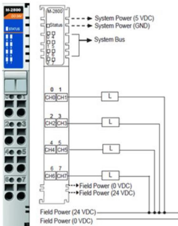
**M-2801: 8 digital outputs, source type, 24 VDC, 0.5 A**
