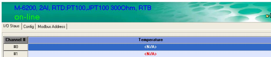
To check the Modbus Address, click on the "Modbus Address" tab.
