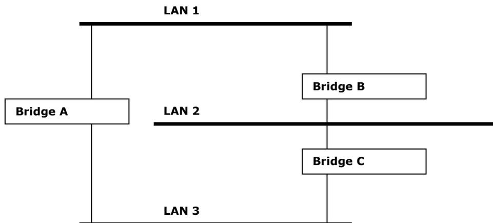
The figure below shows a network made up of three LANs separated by three bridges. Each segment uses at most two paths to communicate with the other segments. Since this configuration can give rise to loops, the network will overload if STP is NOT enabled.
