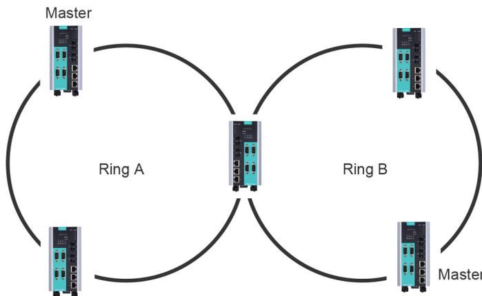
**Dual-Homing Configuration (applies only to “Turbo Ring V2”)**
