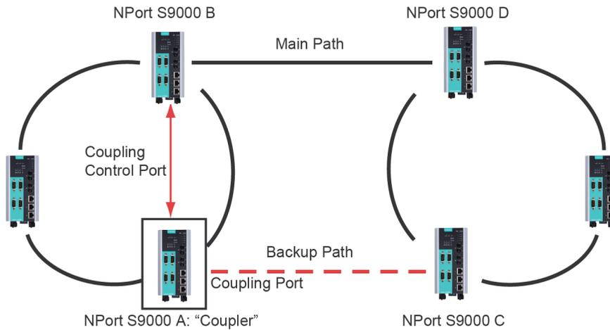
To configure the Ring Coupling function for a “Turbo Ring” ring, select two NPort S9000 devices (e.g., Device A and B in the above figure) in the ring, and another two NPort S9000 devices in the adjacent ring (e.g., Device C and D).
