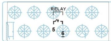
**FAULT:** The relay contact of the 10-pin terminal block connector is used to detect user-configured events. The two wires attached to the RELAY contacts form an open circuit when a user-configured event is triggered. If a user-configured event does not occur, the RELAY circuit will be closed.
