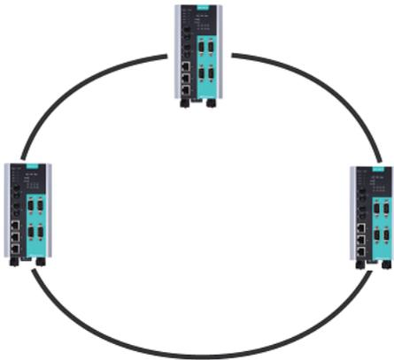
1. For each NPort S9000 in the ring, select any two ports as the redundant ports.
