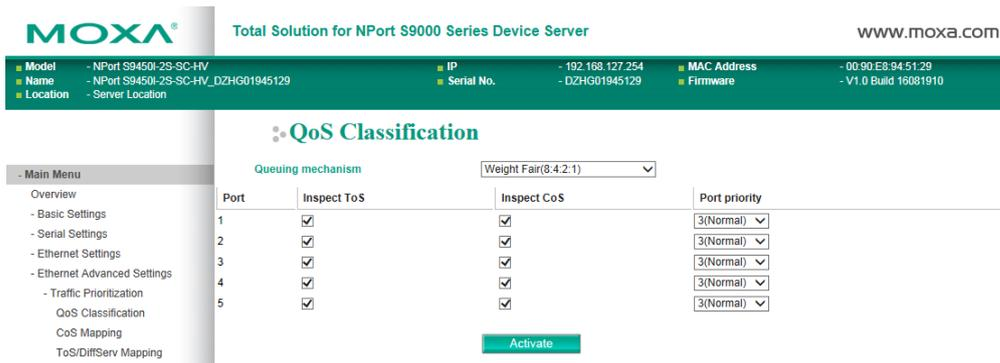
The NPort S9000 supports inspection of layer 3 TOS and/or layer 2 CoS tag information to determine how to classify traffic packets.
