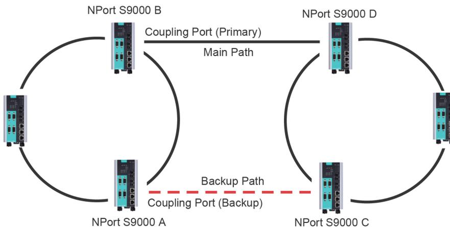
Note that the ring coupling settings for a “Turbo Ring V2” ring are different from a “Turbo Ring” ring. For Turbo Ring V2, Ring Coupling is enabled by configuring the **Coupling Port (Primary)** on Switch B, and the **Coupling Port (Backup)** on Switch A only. You do not need to set up a coupling control port, so that a “Turbo Ring V2” ring does not use a coupling control line.
