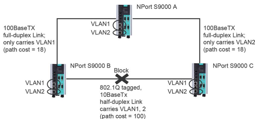
To avoid subdividing VLANs, all inter-switch connections should be made members of all available 802.1Q VLANs. This will ensure connectivity at all times. For example, the connections between Switches A and B, and between Switches A and C should be 802.1Q tagged and carrying VLANs 1 and 2 to ensure connectivity. See the “Configuring Virtual LANs” section for more information about VLAN Tagging.
