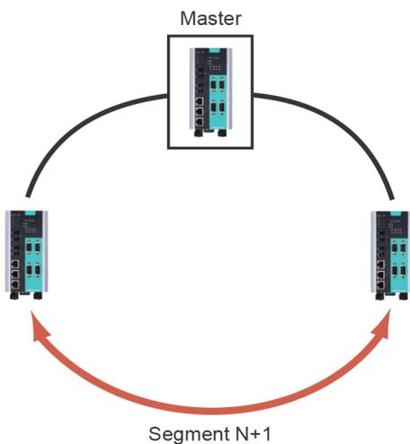
If there are  $2N+1$  NPort S9000 (an odd number) in the “Turbo Ring” ring, with the NPort S9000 and segments labeled counterclockwise, then segment  $N+1$  will serve as the backup path.
