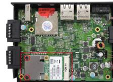
2. Next you need to install the antenna cable. There are two antenna connectors on the Wi-Fi module. Connect the cable onto either connector.
