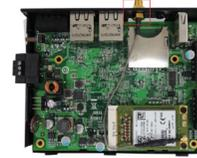
5. Install the connector, place the locker washer first, and then insert the nut. Connect the antenna onto the connector.
