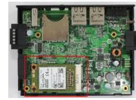
3. Next you need to install the antenna cable. There are two antenna connectors on the cellular module. Connect the cable onto either connector.
