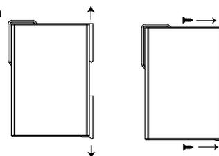
Another method for wall mounting installation is to use the optional wall mounting kit. Attach two mounting brackets on the side panel of the computer, and fasten with screws. Install the computer on a wall or cabinet by fastening two screws for each bracket.
