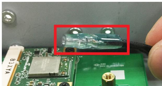
5. Connect the antenna cables to the antenna connectors.
