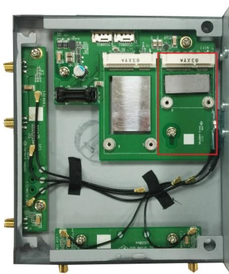
2. Remove the two silver screws on the socket.
