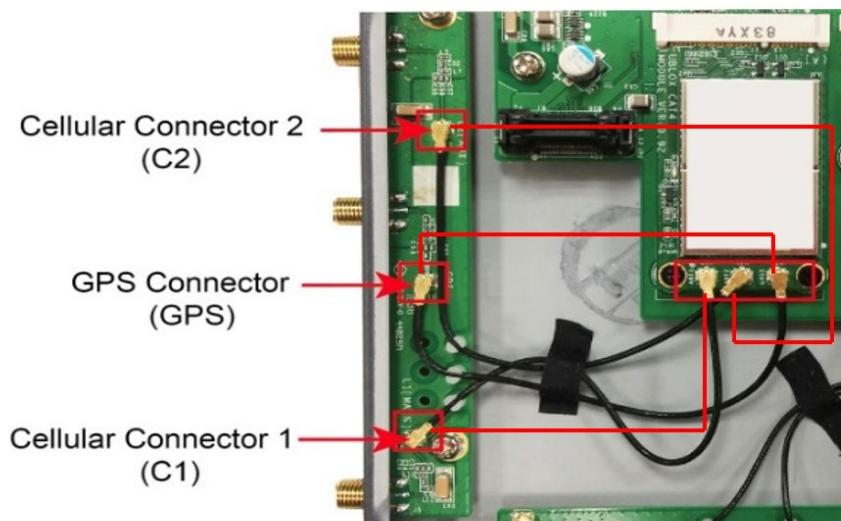
6. The UC-8220 Series supports two cellular antennas and a GPS antenna. Connect the cables to the correct antenna connectors.
