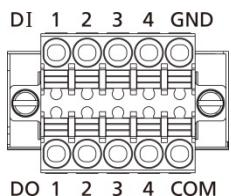
There are four digital inputs and four digital outputs on the top panel. Refer to the figure on the left for detailed pin definitions.
