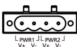
Connect the power jack (in the package) to the UC-8200 Series' DC terminal block (located on the top panel), and then connect the power adapter. It takes about 30 seconds for the system to boot up. Once the system is ready, the Power LED will light up. Both models support dual power inputs for redundancy.
