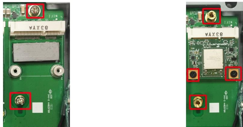
4. Remove the plastic protection covers on the antenna connectors.
