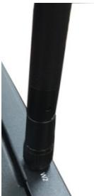
There are two Wi-Fi antenna connectors (W1 and W2) on the top panel of the UC-8220 Series. Connect the antennas on the connectors as shown below. Both W1 and W2 connectors are of RP-SMA type.
