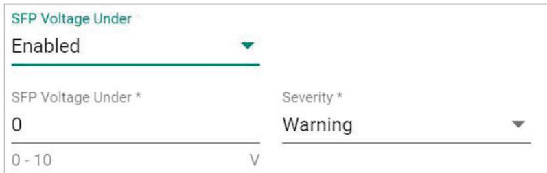
The screenshot shows a configuration form for 'SFP Voltage Under'. The first dropdown menu is set to 'Enabled'. Below it, the 'SFP Voltage Under \*' field has a value of '0' and a range of '0 - 10' with the unit 'V'. To the right, the 'Severity \*' dropdown menu is set to 'Warning'.
