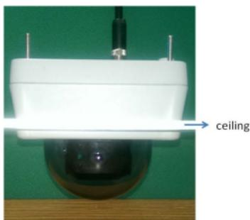
**NOTE** Because of the anti-vibration design, for onboard environments 8 kgf-cm torque is required for all mounting screws.
