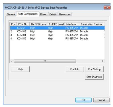
3. Check the Auto Enumerating COM Number option to map subsequent ports automatically. The port numbers will be assigned in sequence. Select Interface (RS-232, RS-422, RS-485-2W, or RS-485-4W) from the drop-down box. An Auto Tuning function is provided with RS-485-2W. Click OK to save the settings.
