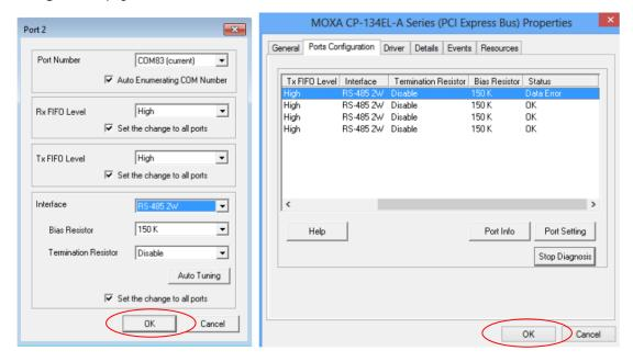
7. Test if the communication is **OK**. If it's not OK, proceed to Step 8.
