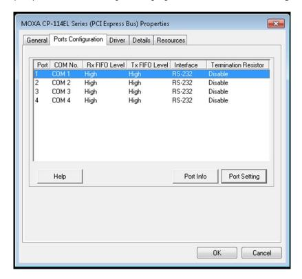
2. Select a COM number for the port from the Port Number pull-down list. Select the **Auto Enumerating COM Number** option to map subsequent ports automatically. The port numbers will be assigned in sequence. For example, if COM 1 is assigned to Port 1, then COM 2 (if not already occupied) will be assigned to Port 2, etc.
