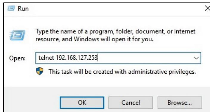
12. Log in to the Telnet console using the default login name **admin** and password **moxa**. This password will be required to access any of the consoles (web, serial, Telnet).
