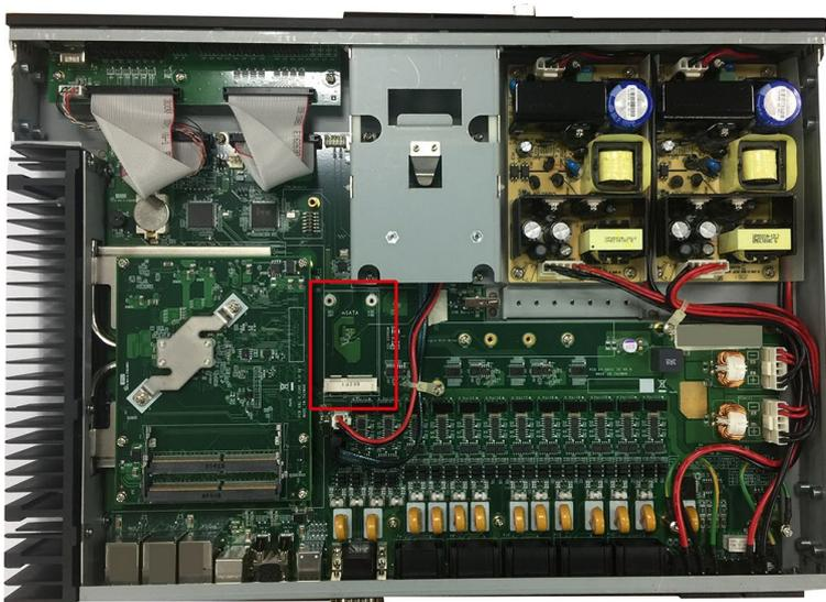
4. Insert the mSATA storage card into the slot and fasten the two screws to secure the card to the slot.
