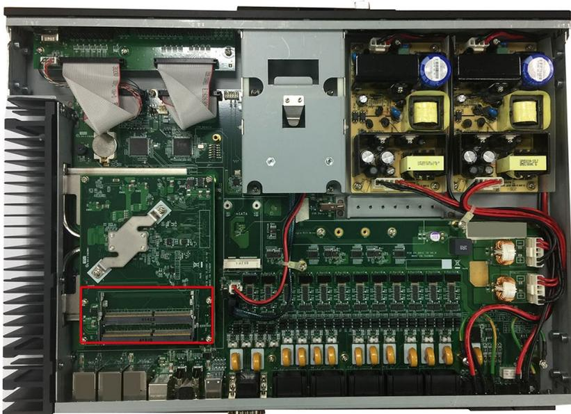
4. Install the new memory module in the slot.
