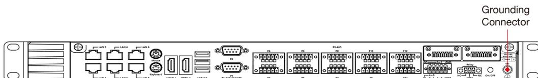
Connect this grounding connector on the chassis to the earth (ground). The minimum wire diameter is 18 AWG.
