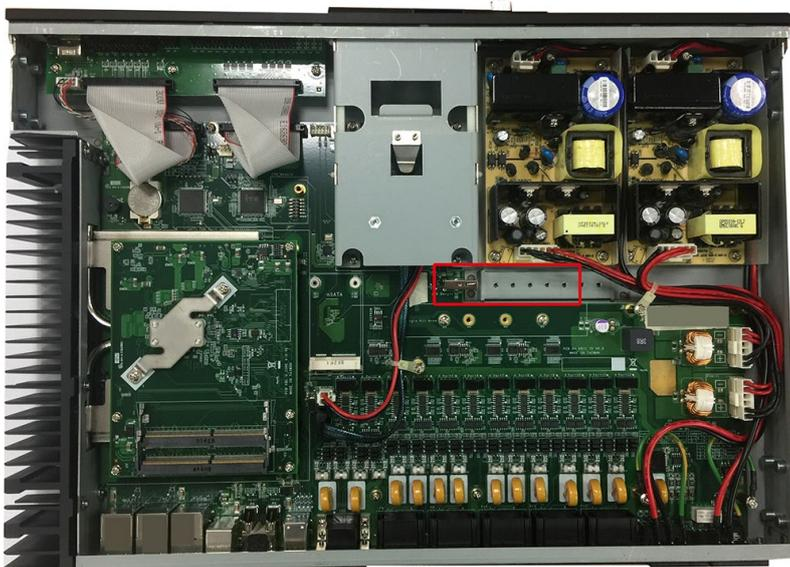
3. Insert the USB device into the USB port inside the DA-681C computer.
