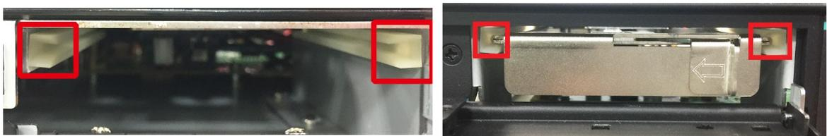
6. Slide the storage slot cover back and fasten the screws to secure it.
