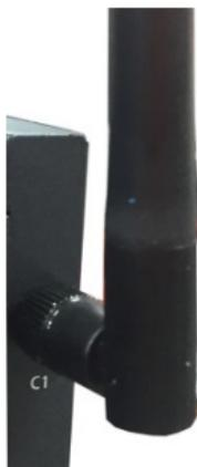
There are two Wi-Fi antenna connectors (W1 and W2) on the top panel of the UC-8220 Series. Connect the antennas on the connectors as shown below. Both W1 and W2 connectors are of RP-SMA type.
