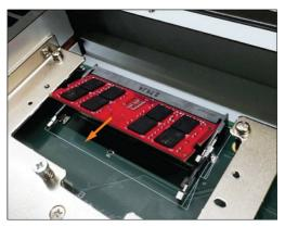
8. Replace the heat sink and the top cover, and fasten all screws.
