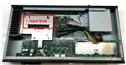
4. Remove the two M3x6 mm screws on the heat sink and remove the heat sink to reveal the memory slot.
