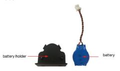
Place a new battery in the battery holder, replace the metal plate, and fasten the two screws on to the frame to secure the battery.
