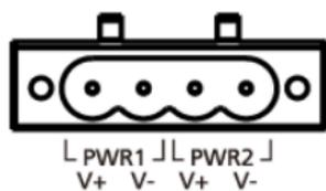
Connect the power jack (in the package) to the UC-8200 Series' DC terminal block (located on the top panel), and then connect the power adapter. It takes about 30 seconds for the system to boot up. Once the system is ready, the Power LED will light up. Both models support dual power inputs for redundancy.
