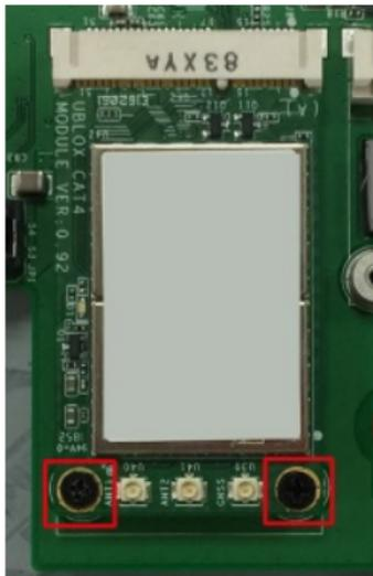
5. Connect the antenna cables to the antenna connectors.
