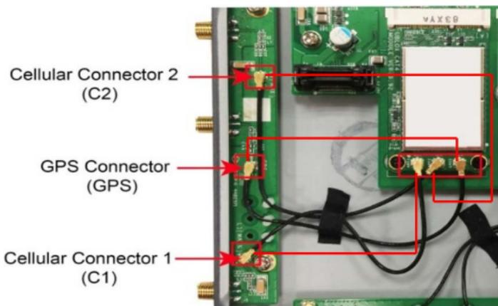
6. The UC-8220 Series supports two cellular antennas and a GPS antenna. Connect the cable to the correct antenna connectors.
