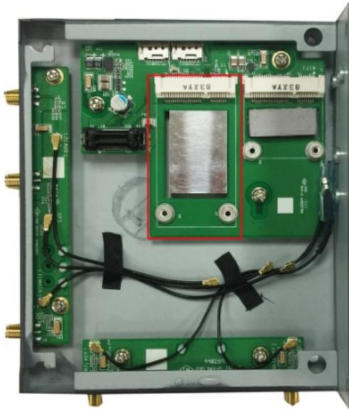
4. Install the cellular module onto the socket and fasten the two screws on the module.
