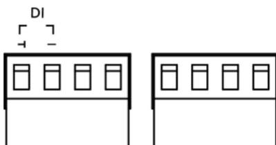
**STEP 1:** Insert the negative (ground)/positive DI wires into the  $\pm$ /I terminals, respectively.
