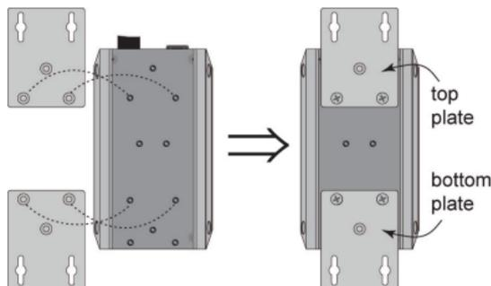
**STEP 2:** Mounting the EDS-G500E series on the wall requires 4 screws. Use the EDS-G500E series, with wall mount plates attached, as a guide to mark the correct locations of the 4 screws. The heads of the screws should be less than 6.0 mm in diameter, and the shafts should be less than 3.5 mm in diameter, as shown in the figure on at right.
