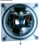
2 screws for fixing the lens in a horizontal position (5.5 kgf-cm)
