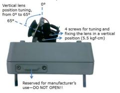
4 screws for tuning and fixing the vertical lens position:
