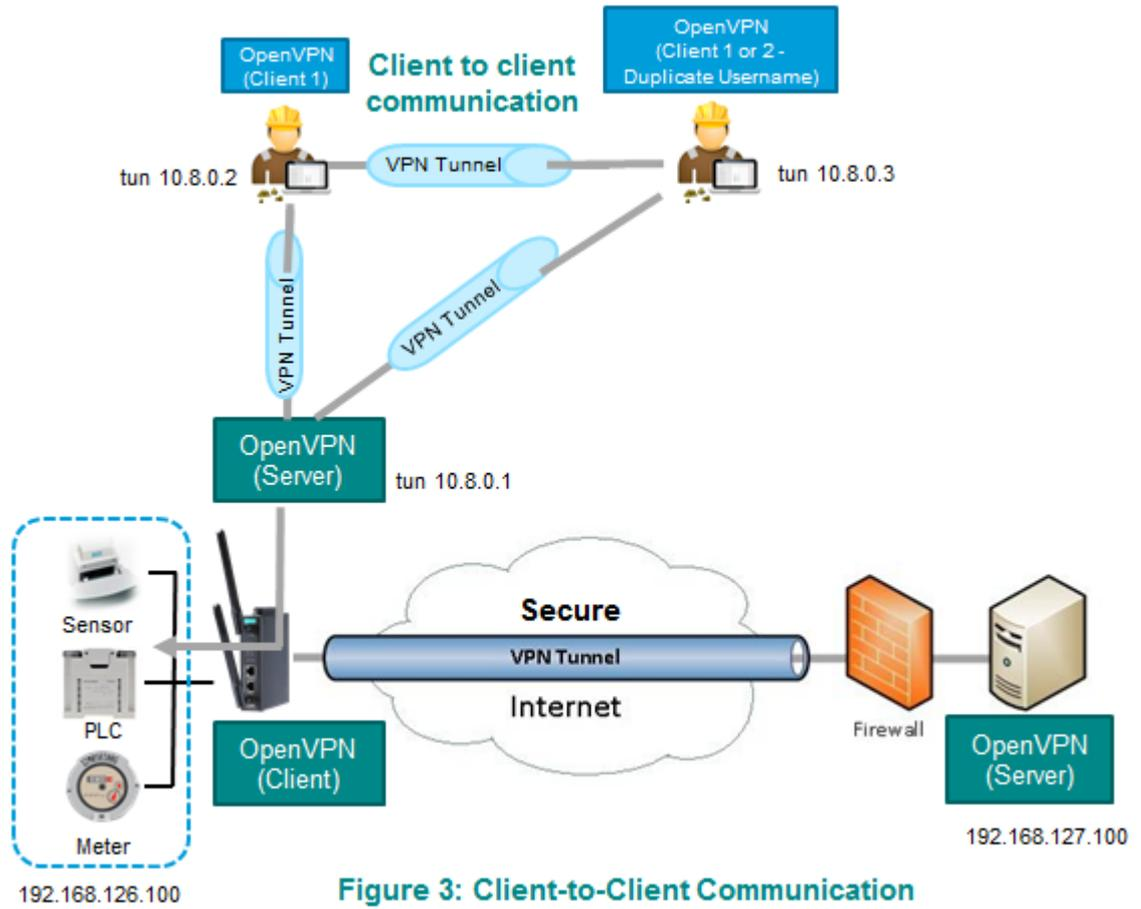
Figure 3: Client-to-Client Communication
