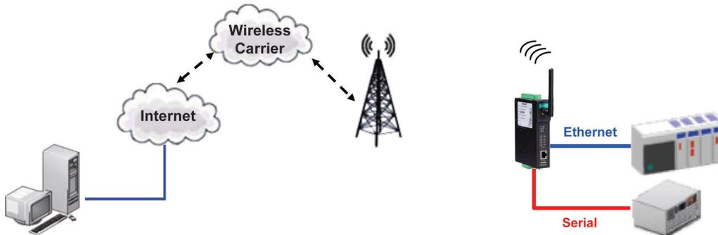
The OnCell 3120-LTE-1 enables traditional serial (RS-232/422/485) devices for transmitting data over the cellular network. The IP gateway can bi-directionally translate data between the serial and IP formats. With the OnCell 3120-LTE-1, your computer will be able to access, manage, and configure remote facilities and equipment over the cellular network from anywhere in the world.
