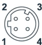
**NOTE** To connect the VPort P06HC-1V to a network, use an Ethernet cable with D-code M12 connector and an M12 PoE switch or RJ45 PoE switch.
