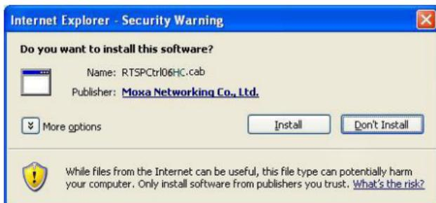
**NOTE** For Windows XP SP2 or later operating systems, the ActiveX Control component will be blocked for system security reasons. In this case, the VPort's security warning message window may not appear. You should unlock the ActiveX control blocked function or disable the security configuration to enable the installation of the VPort's ActiveX Control component.
